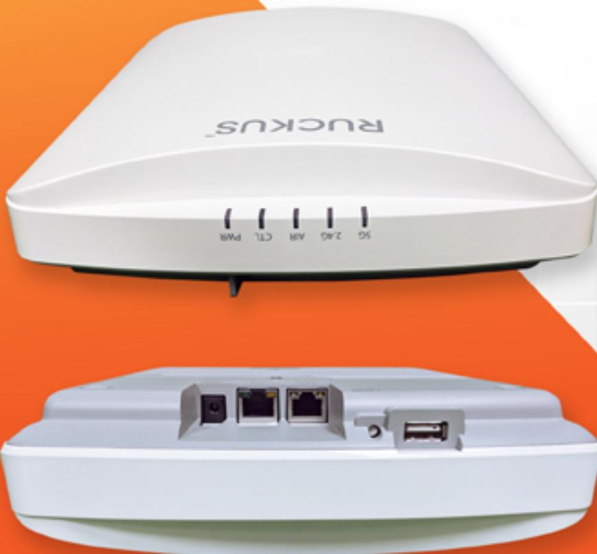
The [Ruckus R750](#) is a dual-band, dual-concurrent Wi-Fi 6 AP that supports eight spatial streams (4x4:4 in 5GHz, 4x4:4 in 2.4GHz), 3.5 gigabit-per-second (Gbps) aggregate throughput and embedded Bluetooth Low Energy (BLE) and Zigbee radios. It serves 1,024 concurrent users.
